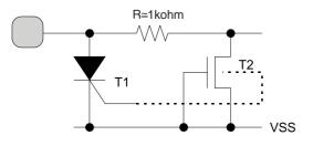
The triac T1 is activated by the **substract** current of transitor T2 when the pad tension strongly increases (ESD pulse).
